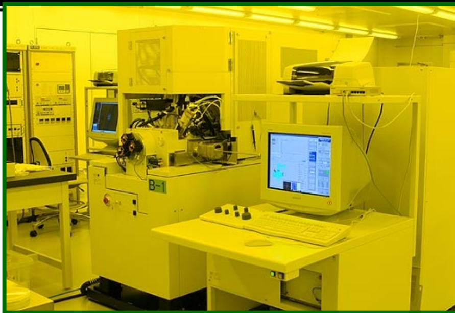
FIB (Seiko Instruments SMI2050, ISIR, Osaka Univ.)
